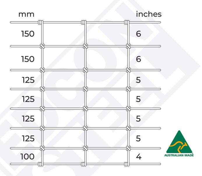
Made from high quality, heavy galvanised fencing wire, FarmFence™ uses the improved version of the old ring joint knot which prevents the vertical wire from slipping along the horizontal wire. The FarmFence™ also has a one piece vertical wire, giving the fence greater vertical stability. These two factors ensures FarmFence<sup>™</sup> is both easy to strain and low maintenance, saving time and money.
