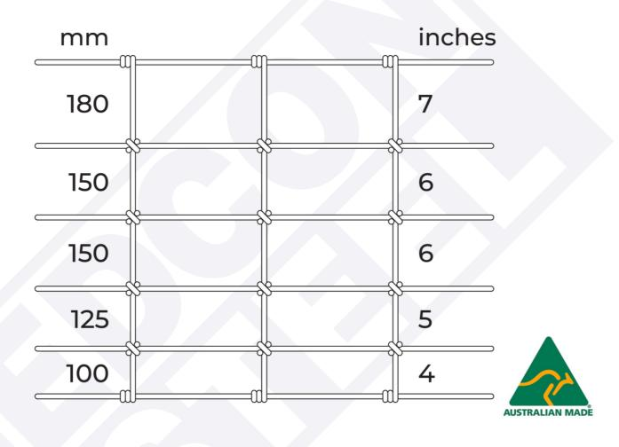
Made from high quality, heavy galvanised fencing wire, FarmFence™ uses the improved version of the old ring joint knot which prevents the vertical wire from slipping along the horizontal wire. The FarmFence™ also has a one piece vertical wire, giving the fence greater vertical stability. These two factors ensures FarmFence™ is both easy to strain and low maintenance, saving time and money.
