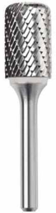
All Bordo burrs are CNC machined for consistently high quality, and offering the latest cut technology, the new Corner Radius Burrs are suitable for use on a wide range of metals, alloys and other materials including titanium, bronze, stainless steel, cast iron and brass. Manufactured and inspected to strict standards from sintered tungsten carbide, its novel design cuts better and lasts longer, giving you a more cost effective and efficient solution for difficult to machine materials.
