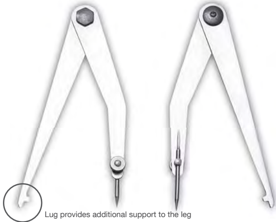
Lug provides additional support to the leg
