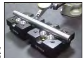
Ball Bearing Vee Blocks with non marring balls being used to check the roundness of a stepped rod
