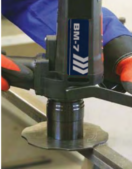
Straight edge bevelling with radius
