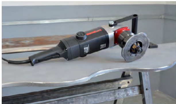
Arched edge bevelling with radius
