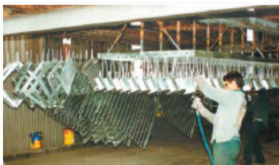
The mass of steel items that can fit on a galvanizing jig is a major factor in costing. These small items have a high cost factor because of the low dip weight and large amount of handling required in processing them.
