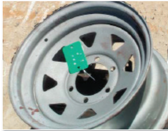
Items are individually tagged for identification. The metal tag remains attached throughout the galvanizing process.
