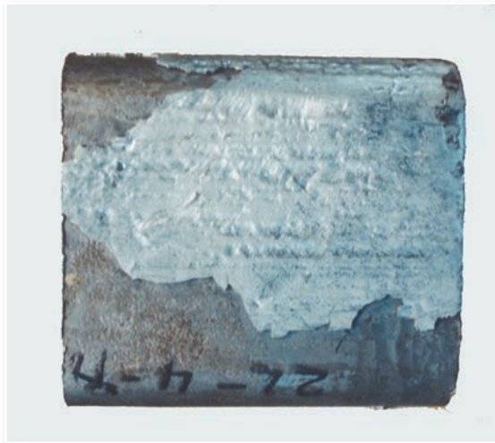
This small RHS section has severe galvanized coating delamination arising from very high phosphorous levels in the steel, creating a thick, fragile coating almost 1000 microns in thickness.
