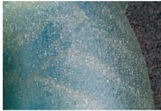
Dross pimples on this pipe spool arise from dross crystals being stirred up from the bottom of the galvanizing bath by long or deep items. Appearance is unsightly but durability is unaffected.
