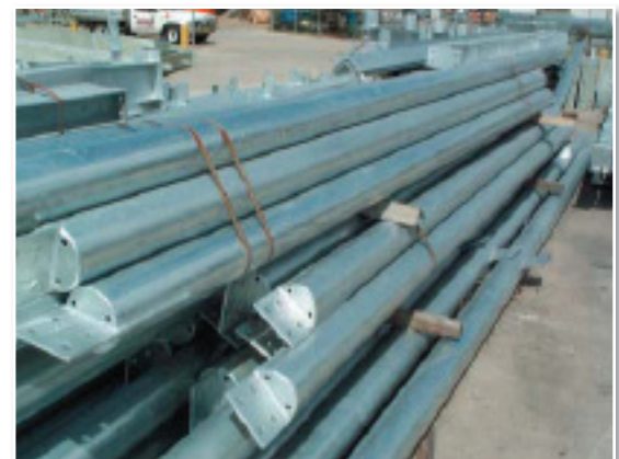
This pipe bracing has been correctly designed with multiple vent and drain holes at each end of the hollow sections.
