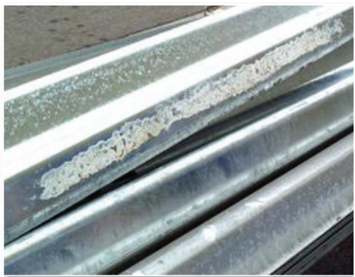
Severe white rust on a galvanized section of guard rail as a result of rails being tightly nested and stored in wet conditions
