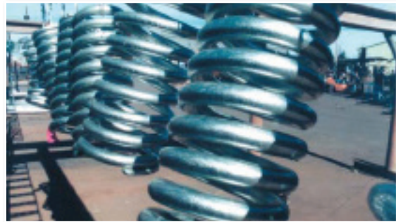
These heavy coil springs have been successfully galvanized following special handling of this high silicon material.
