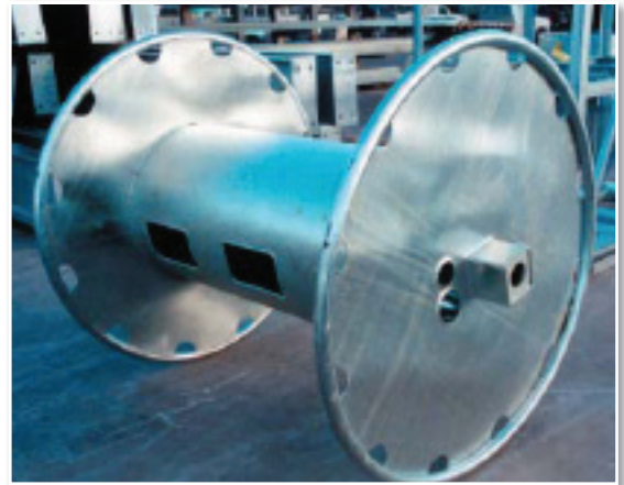
Good design for galvanizing on this cable spool produces a high quality result. All hollow sections are well ventilated and drained, as is the flange rim.
