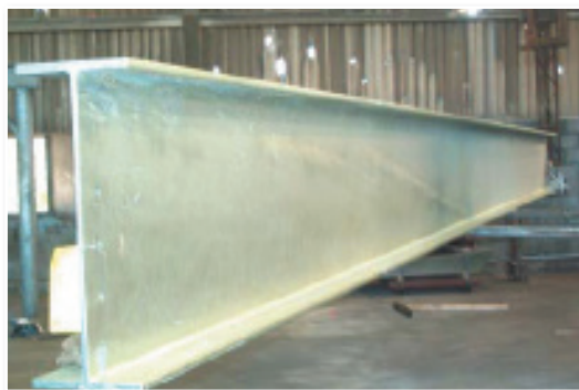
Large and simple structural members such as this universal beam can be galvanized at lower cost because of the ease of handling, the significant mass and relatively low zinc pick up on the heavy section.
