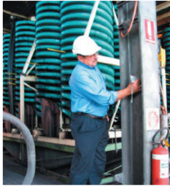
The durability of metallic coatings like hot dip galvanizing are dependent on their coating thickness. Measuring coating loss over time can accurately determine coating life.
