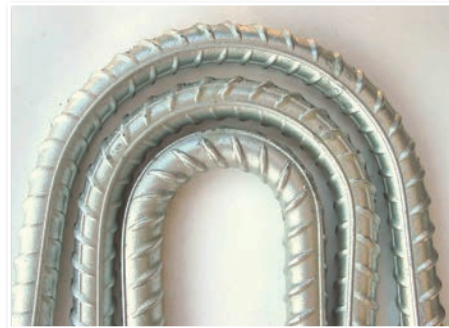
All 500N Grade 32mm reinforcing bar passed the bend test if bent after galvanizing and AS 3600 specifications for bend radii were adhered to.
