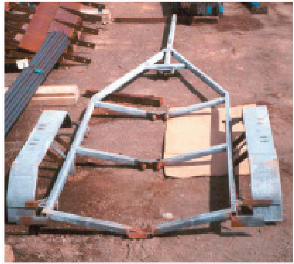
The re-galvanizing of old boat trailers will restore them to 100% original condition. Boat trailers, anchors and chains are routinely re-galvanized to restore their original corrosion prevention performance.
