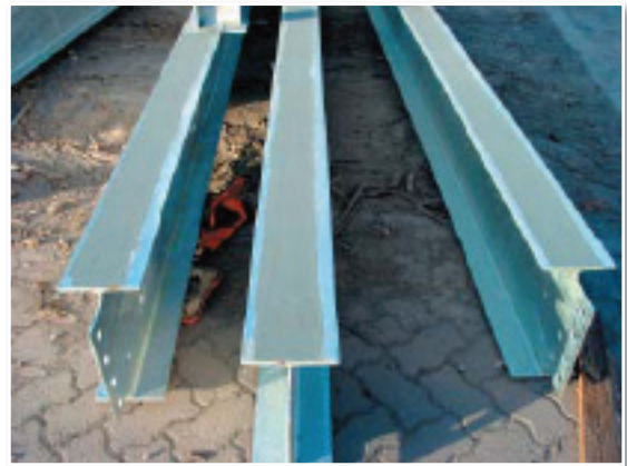
These universal beams have been masked on the top flange to prevent the galvanized coating forming. This has been implemented by the galvanizer to allow shear studs to be welded to the beams on site. The galvanized coating interferes with the resistance welding of these connections.
