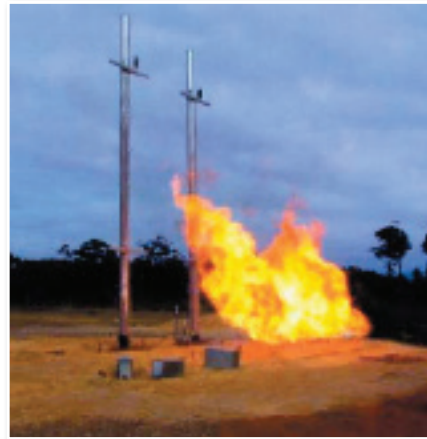
CSIRO Bushfire CRC – Mogo NSW. Sureline galvanized steel poles undergoing Level 2 bushfire testing. This test simulates actual bushfire conditions and flame duration. Galvanized coating unaffected.
