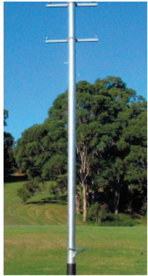
Galvanized steel poles have been direct buried for many years. BlueScope Steel's newly developed Sureline pole is designed for a minimum of 50 years in-ground service, using heavy galvanized coatings and membrane systems at the ground line.
