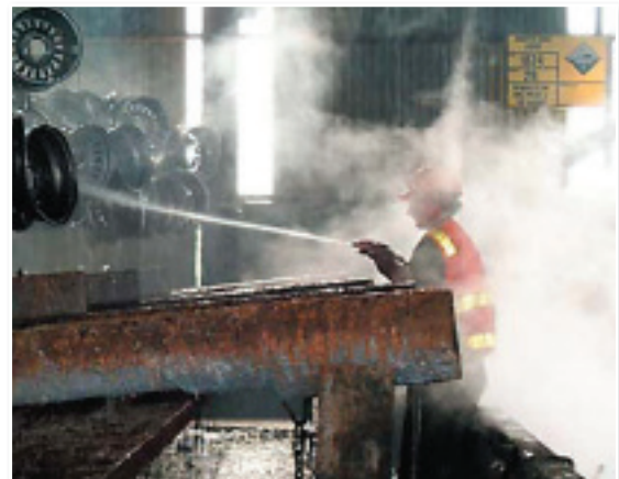
Chemical pre-treatment usually involved multiple processes. This hot caustic degreasing operation in the hot dip galvanizing process is necessary to ensure the acid pickling stage is effective.
