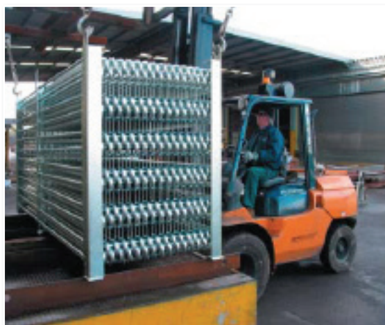
Complex items like this large cooling coil are technically difficult to galvanize, as heavy ballast is required to immerse the tubular assemblies that are full of air, into the molten zinc. Industrial galvanizers has developed special handling equipment to process
