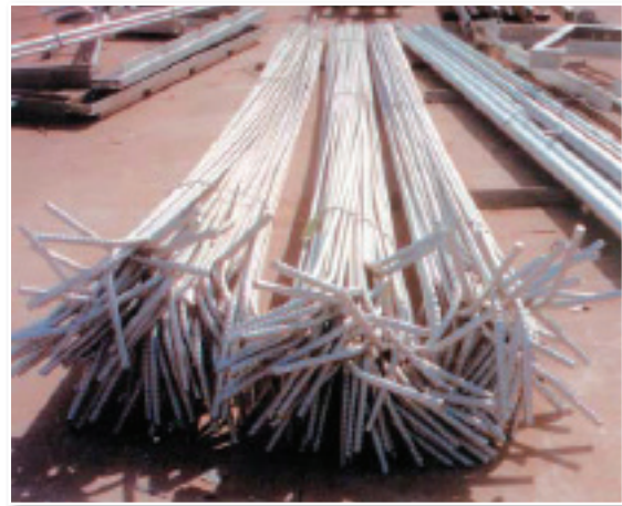
Reinforcing bar in routinely galvanized throughout Australia, where concrete durability is critical
