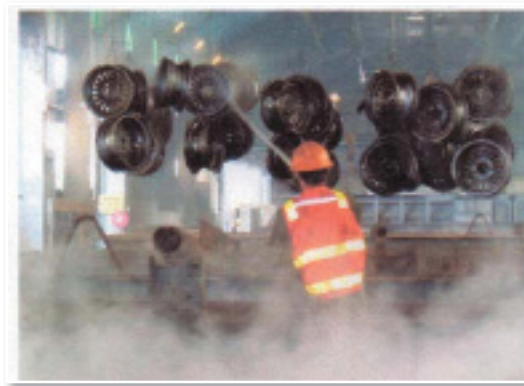
The hot dip galvanizing process uses chemical pretreatment. Close control of the pre-treatment chemistry ensures reliable galvanized coating application.
