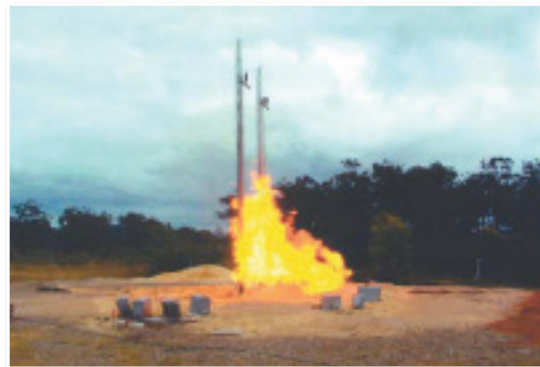
CSIRO Bushfire CRC – Mogo NSW. Sureline galvanized steel poles undergoing Level 3 bushfire testing. This test substantially exceeds actual bushfire conditions. Galvanized coating unaffected
