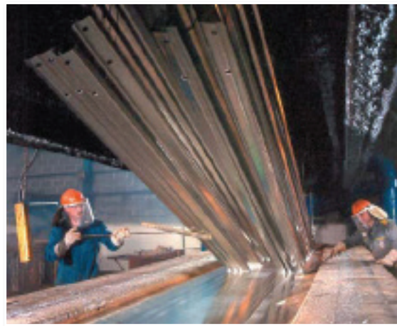
Hot dip galvanizing after fabrication applies a heavy zinc-based coating to a wide range of manufactured products. The zinc-iron alloy layers in the coating provide it with additional abrasion resistance.
