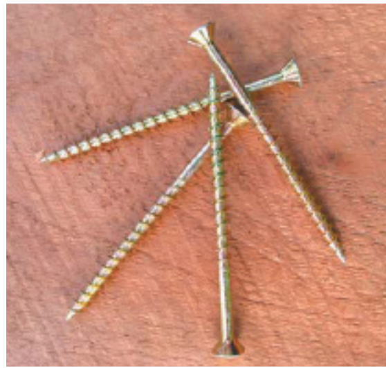
Zinc electroplated coatings are used on a wide range of builders hardware. The relatively thin, pure zinc coating is unsuitable for external applications.
