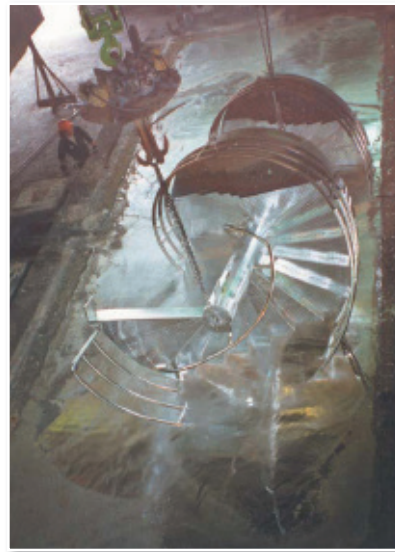
Large fabrications such as this spiral staircase can be hot dip galvanized by double-dipping. The first stage of the process is shown here.
