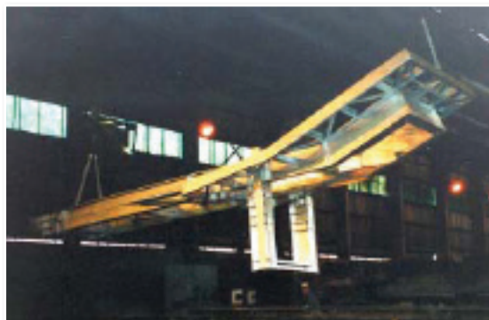
Fabrications like this large frame require double dipping, which is typically 30% higher cost than single dipping because of the extra time in handling.
