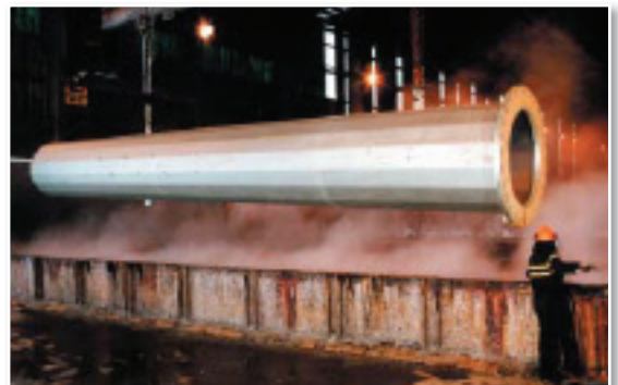
This 10 tonne pole section was galvanized using the heavy lifting capacity of the Industrial Galvanizers' Newcastle plant.
