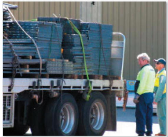
Documentation accompanying fabricated steel deliveries for galvanizing should detail all items in the consignment. The galvanizers describes and tags items after delivery to track items through the galvanizing process.
