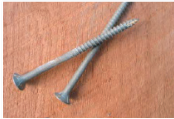
Mechanical plating peens zinc or zinc alloy particles into the steel surface. It is effective on small fasteners where, particularly self-drilling screw where cutting edges must be maintained.
