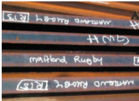
Clearly marked items make processing of loads easier for both client and galvanizer. The correct type of strippable marking paint should be used to ensure removal in the pre-treatment process prior to galvanizing.
