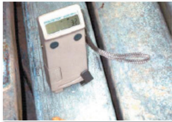
Electronic thickness gauges such as this Positector 6000 can measure any non-magnetic coating over a steel substrate. All coating specifications are based in applied coating thickness.
