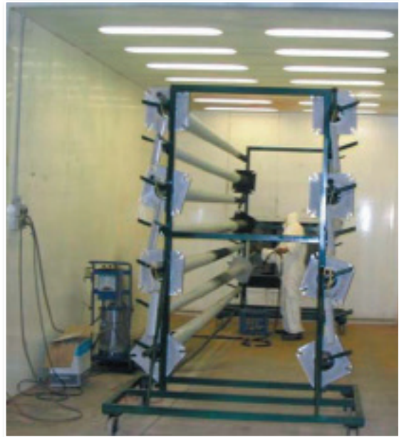
Superior Coaters uses a batch powder coating system for coating all of INGAL EPS' Estate Poles. On-site garnet blasting facilities and large booths and ovens allow the processing of these larger galvanized poles.
