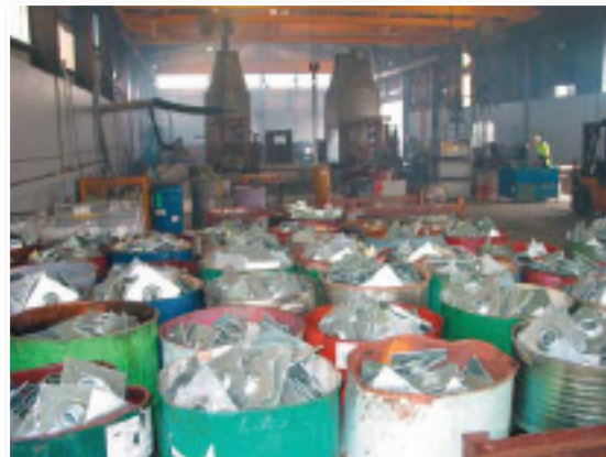
Specialised centrifuge facilities are available in Industrial Galvanizers' plants in Melbourne, Sydney and Brisbane, to process large quantities of small parts for the manufacturing industry in those regions.
