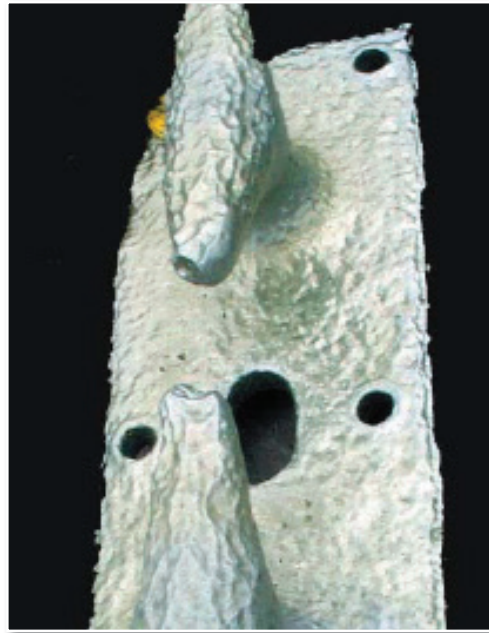
This 50-year old cast marine bollard has been hot dip galvanized. Although it is badly pitted, the bollard was easily re-galvanized to restore its durability.
