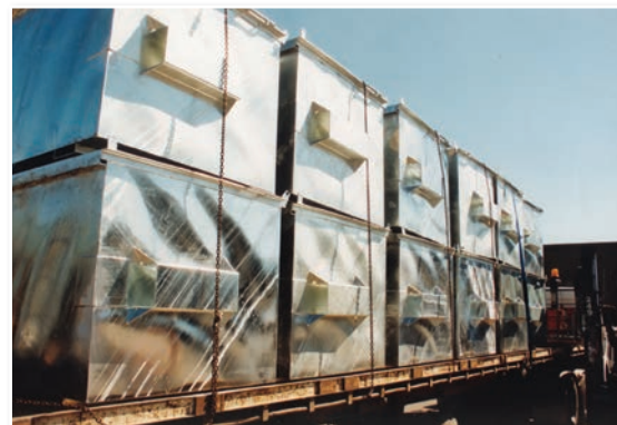
Thin, flat sheet will always buckle in the galvanizing process. Corrugating or ribbing of these type of sections will significantly reduce the likelihood of distortion during galvanizing.
