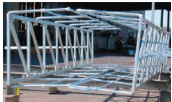
3-D fabrications made up of complex hollow sections require careful design detailing to ensure they can be successfully hot dip galvanized, because of the venting and draining requirements of the individual elements.
